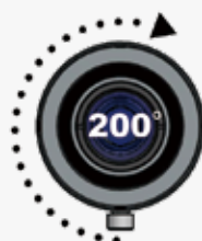
Existing Lens Focus ring rotation angle: 200°
