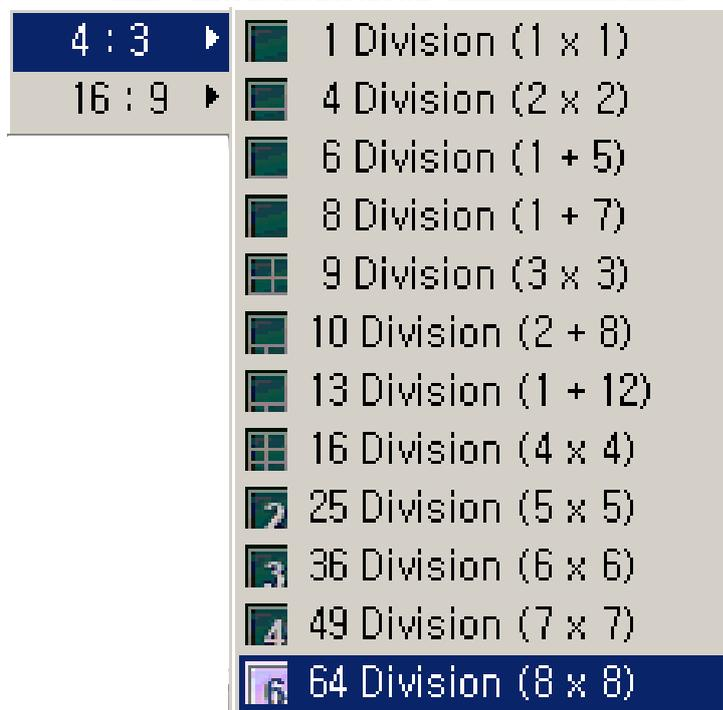
3. Select the required layout for your new view. You are able to select layouts for displaying up to 64 (8x8) cameras in a single view
