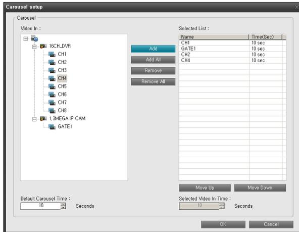
3. If required, move cameras up and down in the list to determine the sequence in which cameras will appear in the carousel.
