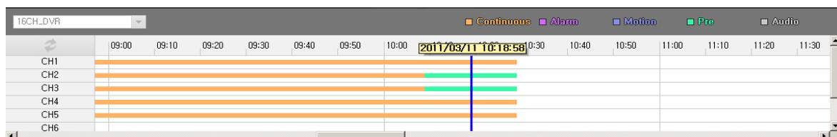
The number of timelines displayed in the timeline browser reflects the number of cameras of device. Cameras with an audio device attached are represented by a double timeline: a timeline displaying periods with video recordings and a timeline displaying periods with audio recordings. Up to 16 cameras can be displayed with audio timelines. If 16 cameras with associated audio are included in the view
