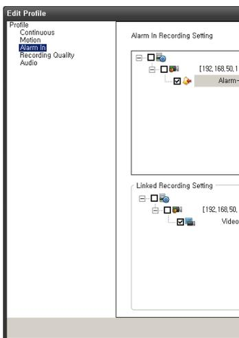
5. Select an Alarm device from device list.
