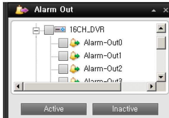
Or user can deactivate the alarm out from the active state of Alarm out by [**Inactive**] button.
