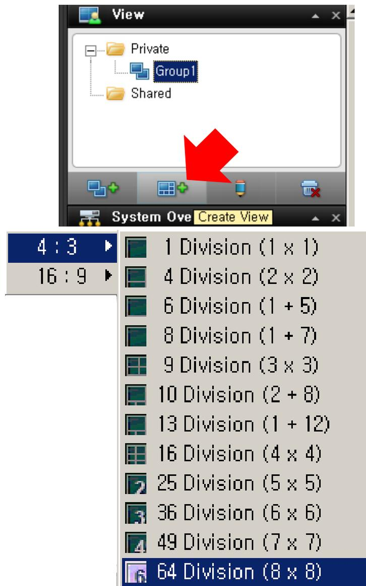
3. Select the required layout for your new view. You are able to select layouts for displaying up to 64 (8x8) cameras in a single view.
