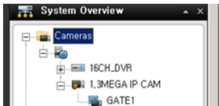
3. Select the required camera from the list, and drag the camera to the required position in the view. When you have dragged a camera to a position in the view, an image from the camera will—provided a connection can be established—appear in the selected position. If a connection cannot be established, for example if the surveillance system's is not on recording mode, the name of the camera will be displayed in the selected position.
