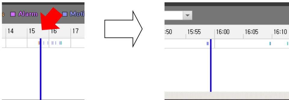
\*The time line can be expanded up to 5 minute term when left click of mouse on time label. Right click of the mouse will compress the time line.
