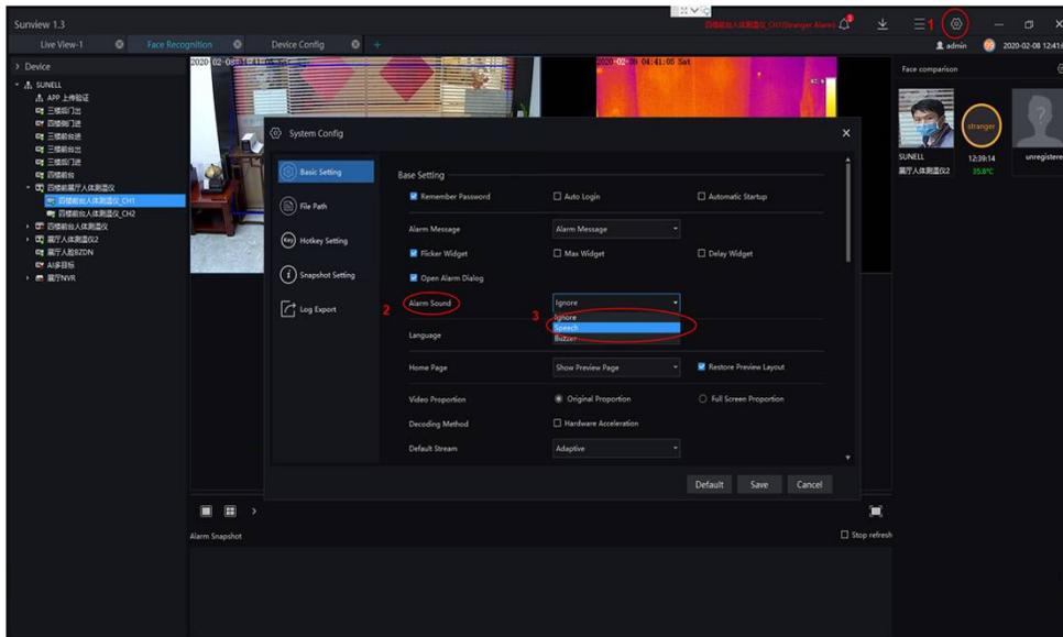
1. Click the button 1 in the figure, enter the system configuration interface, then set the alarm pop-up window and alarm sound.
