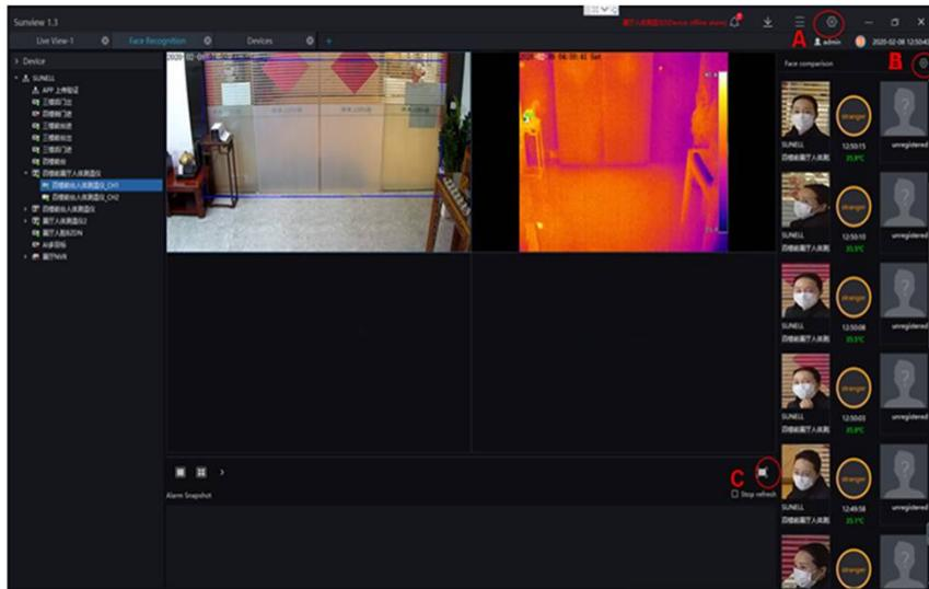
1. The left side of the figure is the device list, the upper middle area is the live video window, the lower middle is the capture area, and the right side is the face comparison and temperature display area.
