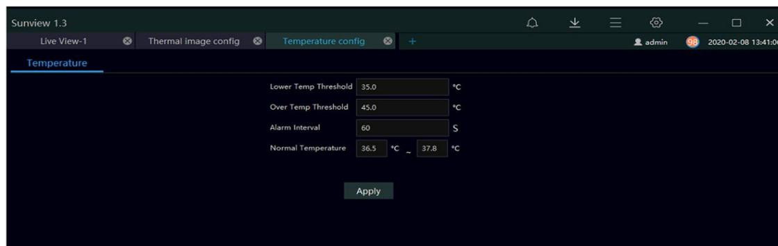
1. On the function page, click the temperature configuration card to enter the temperature configuration interface, as shown above.
